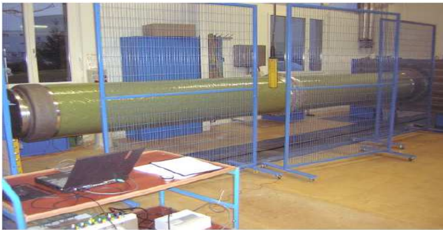
Fig. 1 Bending Test set up
