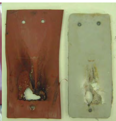
Failure by erosion
